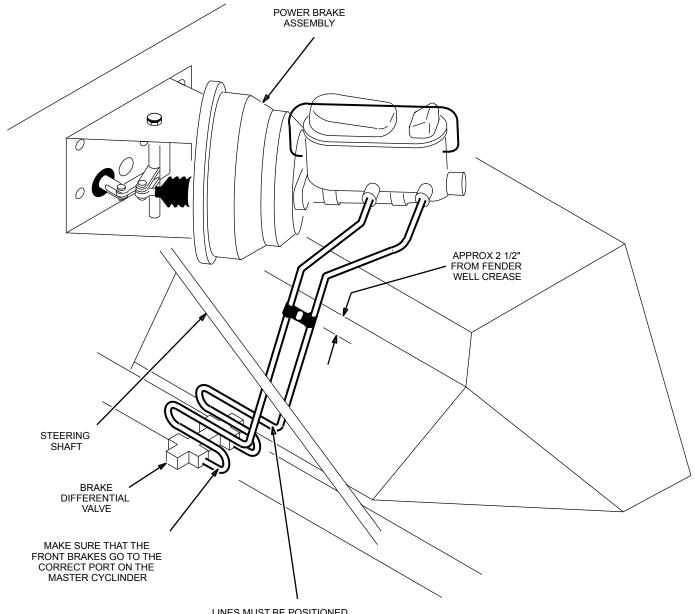
LINES MUST BE POSITIONED BETWEEN FENDER WELL AND STEERING SHAFT.
